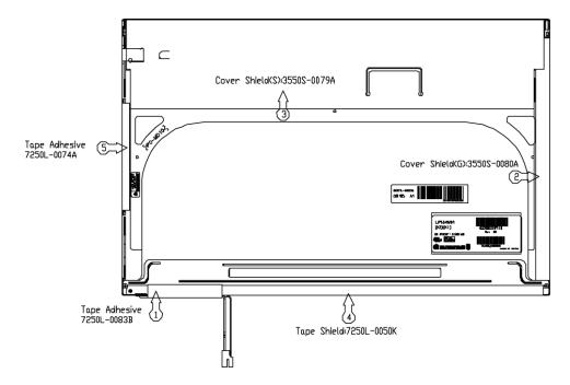
Figure 4-62 Replacing LG.Philips fluorescent lamp (WXGA) (1)
